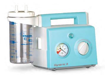
The piston pump guarantees high suction capacity (201/min) and requires no maintenance. With the vacuum regulator, you operate the vacuum size in the range of 0 - 80 kPa. This value is monitored on the vacuum manometer.
