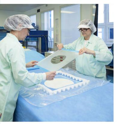
Surgical drape sheets, wear and small sets are packed automatically and undergo EtO sterilization on the premises of DINA-HITEX. This process speeds up the production time considerably. Sterile products are delivered to final users, non-sterile are usually manufactured for B2B contracts.
